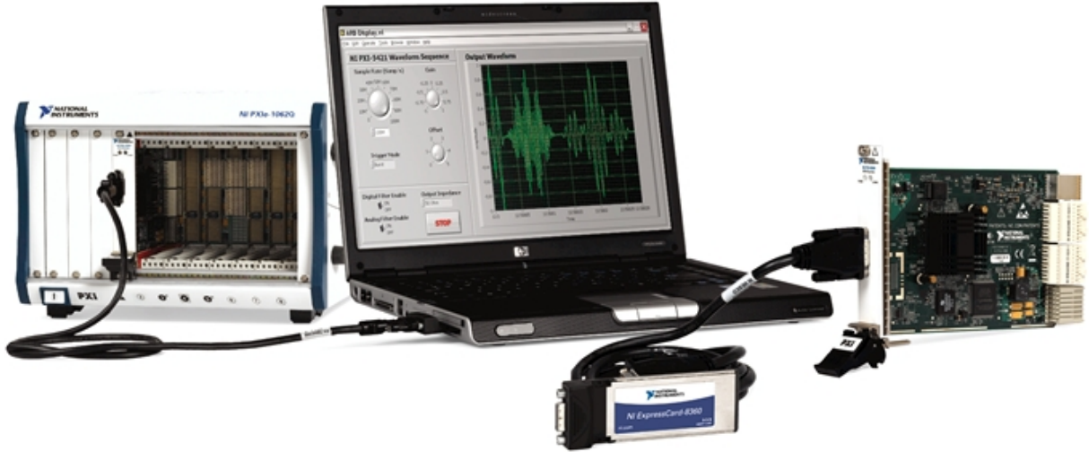
Figure 4. Laptop Control of PXI with NI PXIe-ExpressCard8360 MXI Interface
