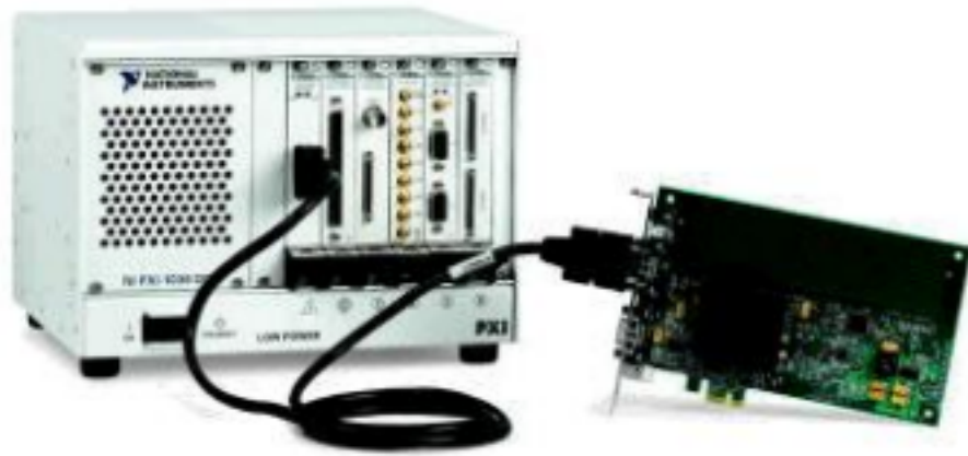
Figure 5. Remote control with two-port MXI-Express provides simultaneous control of two PXI chassis with a combined 838 MB/s throughput.
